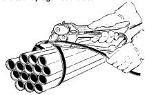
While standing to one side of the strap line, tension the strap with forward and backward motions of the tension handle.
