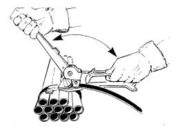
When desired tension is reached, push the drive pawl forward and rotate the tension handle back to contact the lift arm.
