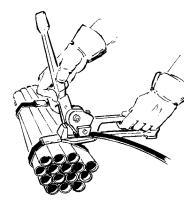
Notch the seal with a Signode sealer to complete the joint.
