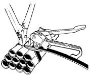
Break off the strap at the seal by repeatedly raising and lowering the tool. Inspect the joint to make sure the seal has been properly notched. Refer to the sealer Service Manual.
